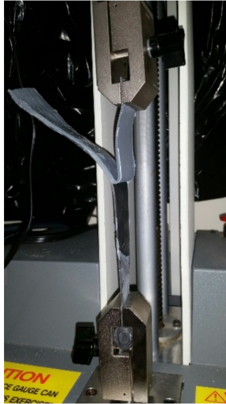
Figure 1 Peel test setup
