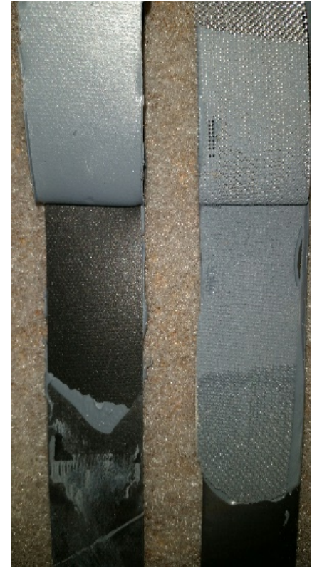
Figure 2 Adhesive failure (L) Cohesive failure (R)
