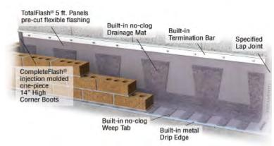
TotalFlash® pre-assembled panels 5-1/2-ft. (5-ft. net) panel
