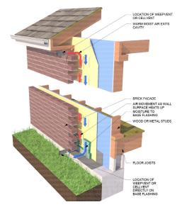
CellVents help ventilate the top and bottom of wall
