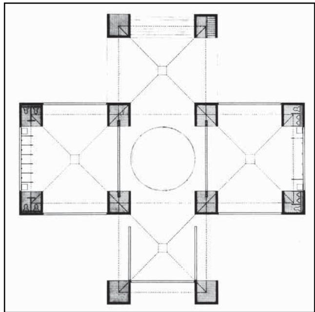
**This image shows the Bath House’s classic “Greek cross” design. In two places, the edges of the suspended roofs are flush with the devising walls beneath them. Kahn envisioned rainwater pouring romantically down the unsealed, unflashed walls. It did—leading to premature wall-failure.**
