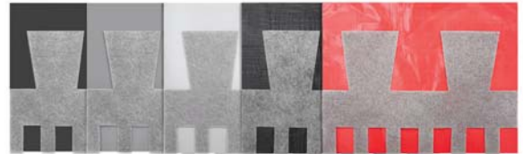
Membrane Materials - (left to right) Ethylene Propylene Diene Monomer (EPDM), Thermoplastic Polyolefin (TPO), Rubberized Asphalt & Copper Laminate
