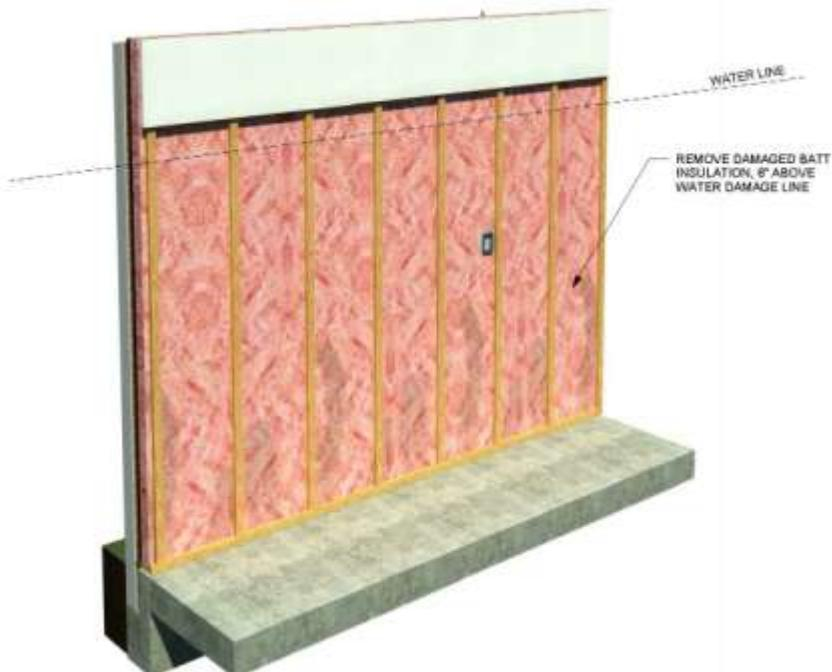
Once the bulk material is removed from the wall, the sheathing that is remaining between the wall ties and the studs, as well as mortar droppings at the base of the wall, can be removed. Any products used to prevent mold would be applied at this point, along with fans to assist and speed the drying time of remaining materials.
