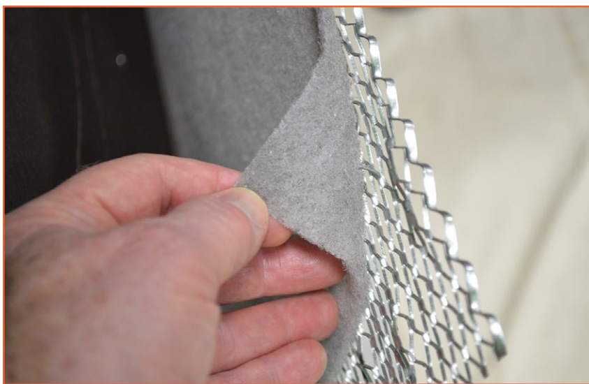
Fig. 2 – Self-furring metal lath with mesh drainage plane.
